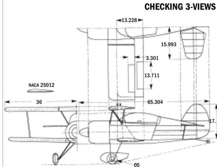
FIG 1 This is my CAD drawing of a 72-inch-span Pitts Model 14. Reference lines are shown to match up height, width and length of the top, side and front views.
