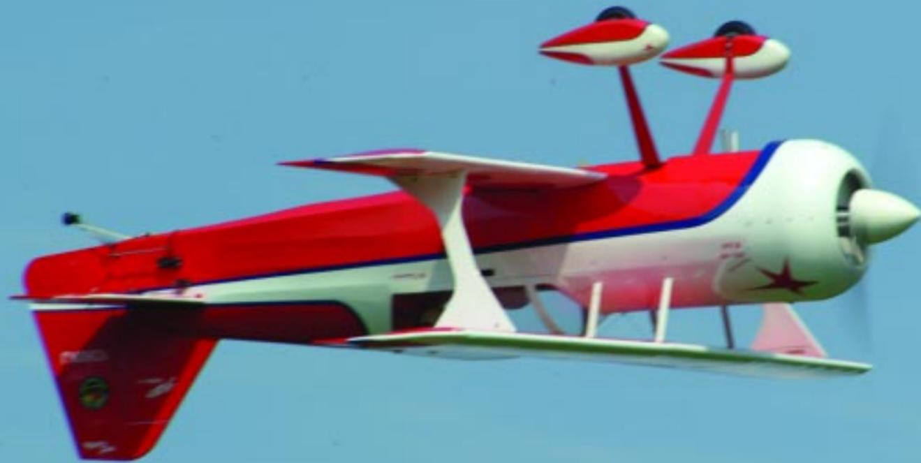
This 41-percent Pitts Model-12 biplane designed by Bob Trueworthy of Bigairplanes.com is a great example of a CAD-designed model. It has a 108-inch span and is powered by a 150cc gas engine. Thanks to the flexibility of CAD, Bob offers a smaller version of the same design.
